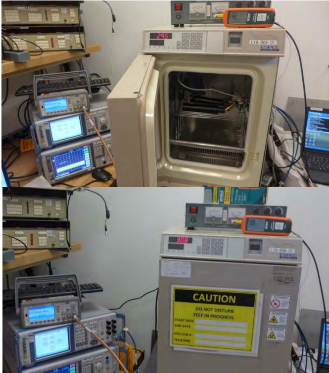
Figure C-1 - Test Setup for Frequency Stability
