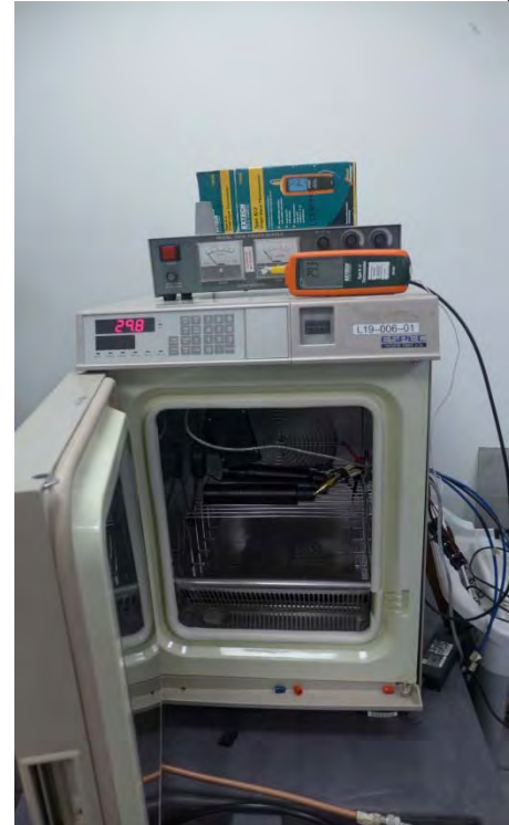
Figure C-1 - Test Setup for Frequency Stability
