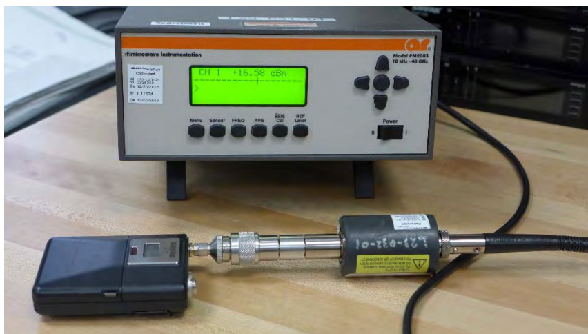
Figure A-1 - Test Setup for RF Power Output
