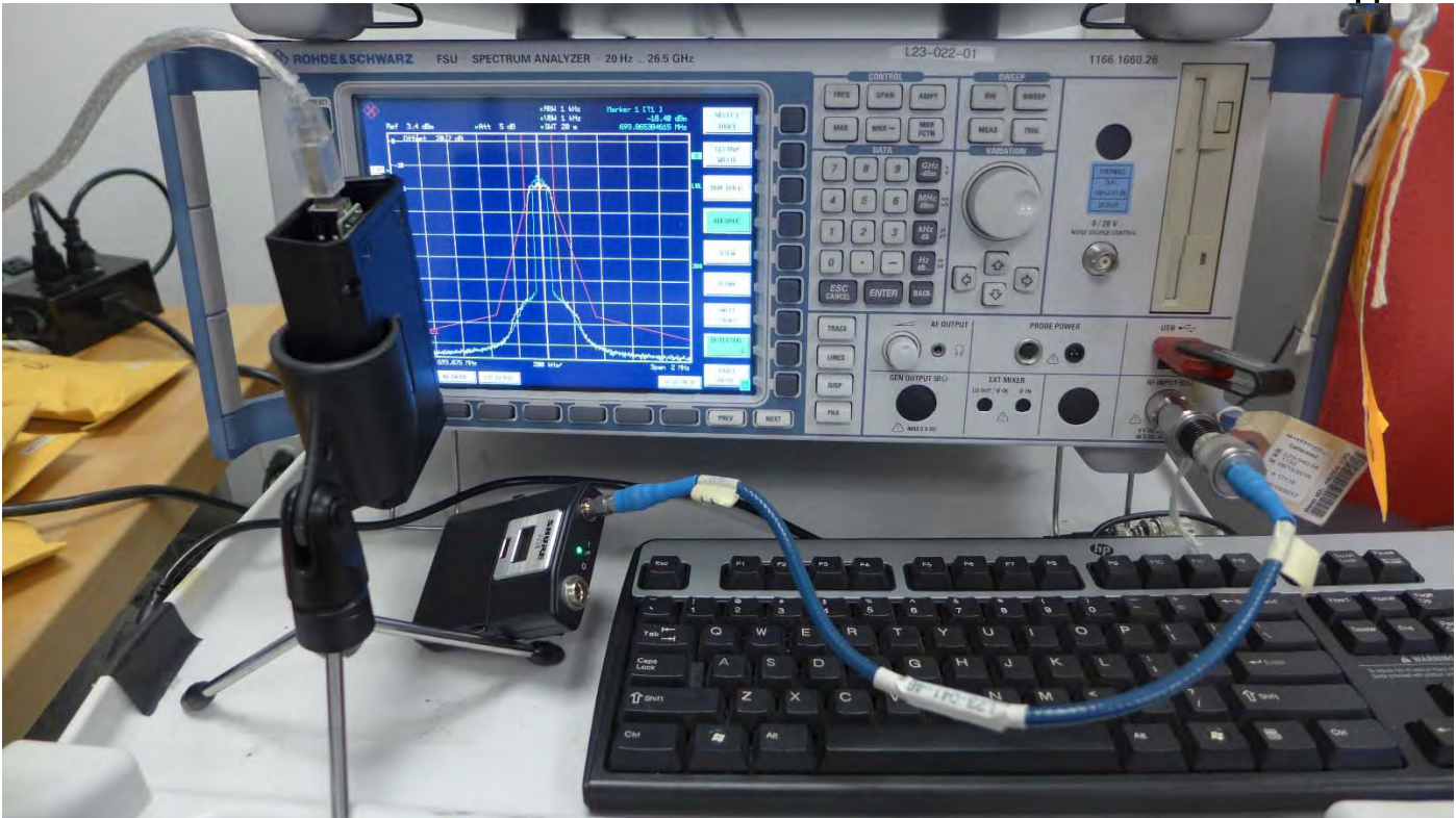
Figure D-1 - Test Setup for Occupied Bandwidth
