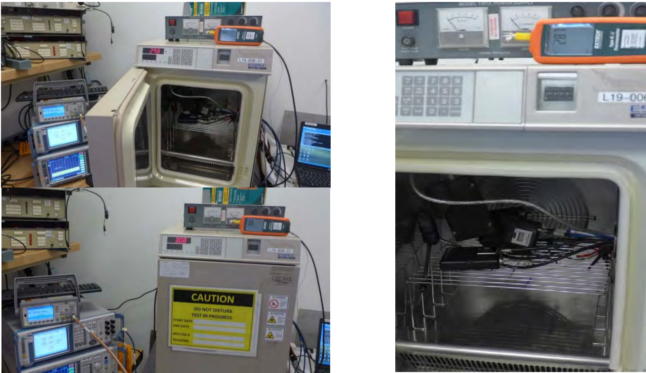
Figure C-1 - Test Setup for Frequency Stability
