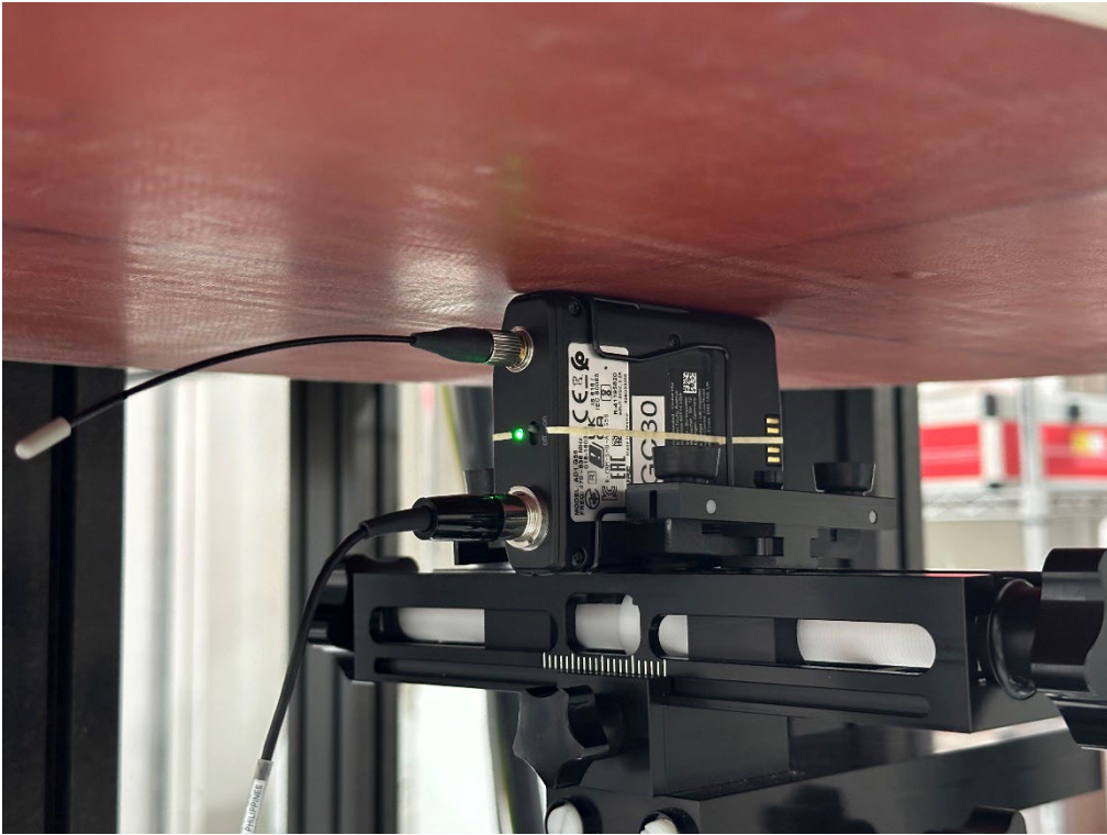
Description: Body Right Position with 0mm gap for G57 Band
