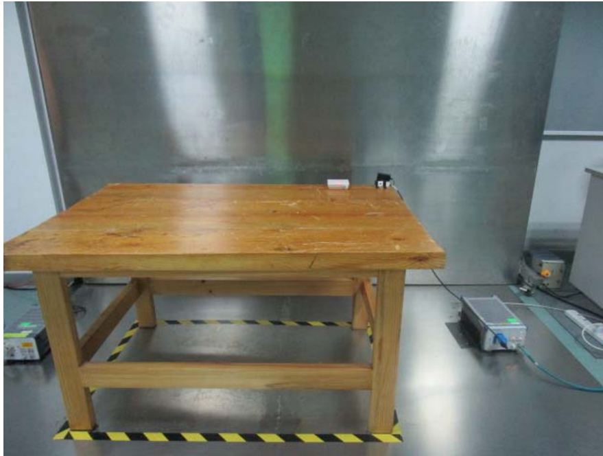
Conducted Emission--Front View (DC 12V)
