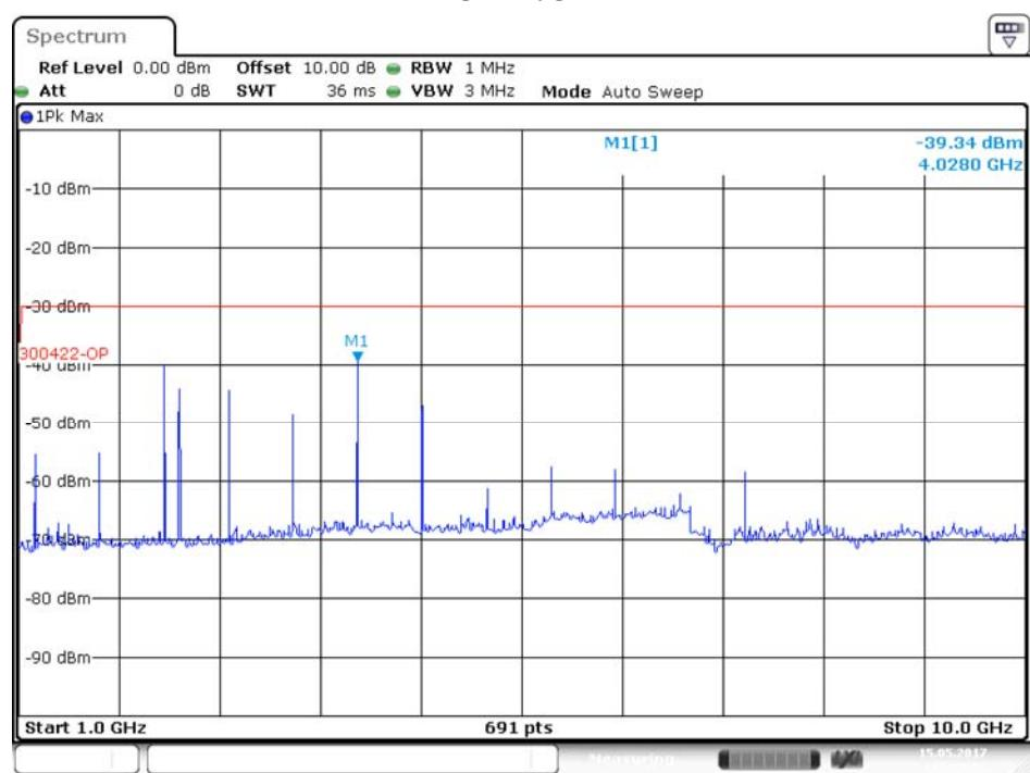
Note: The limit line in above plots is based on EN 300 422 limit; however, FCC limit line is -13 dBm. Plots comply with both FCC requirements
