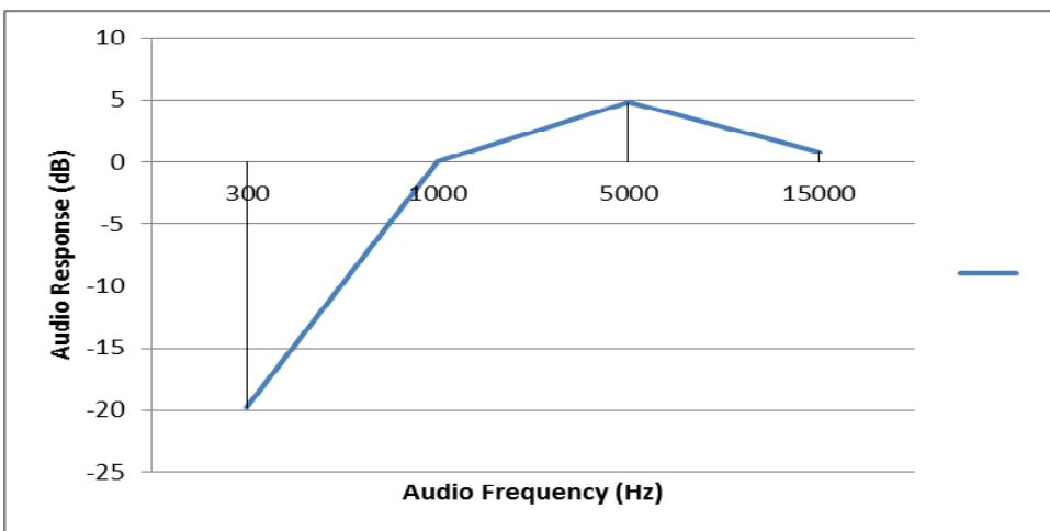
Note: AF Response =  $20 \times \log (\text{AF Level of 1 kHz}/\text{AF Level})$
