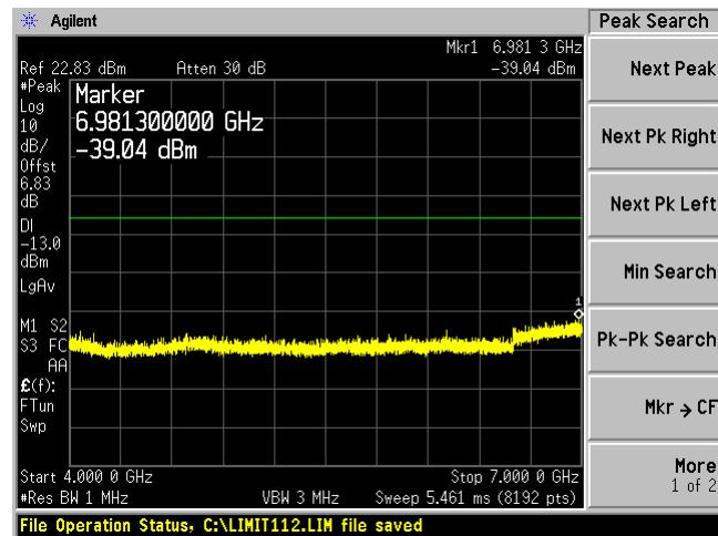
Note: The limit line in above plots is based on FCC limit; however, IC limit line is -25 dBm. Plots comply with both FCC and IC requirements.
