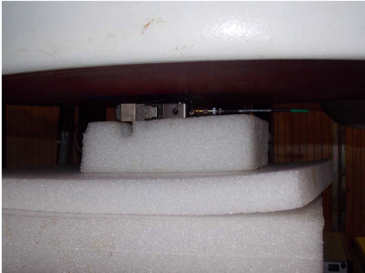
Test Position Back Both Antennas 0 mm Gap
