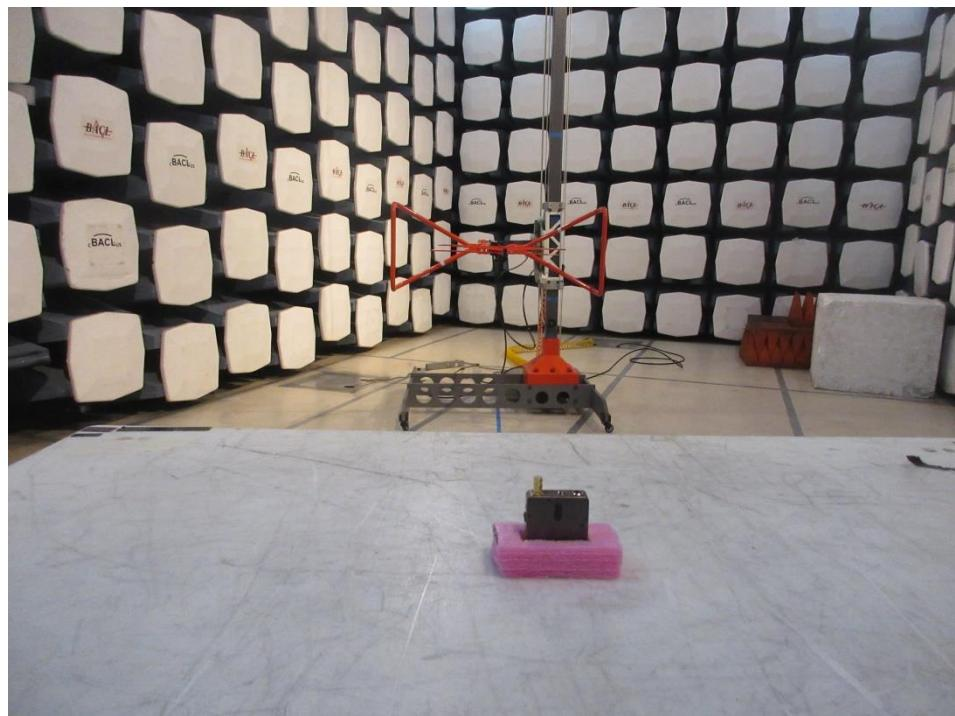
**1.7 Radiated Spurious Emissions: 1-18 GHz Front View at 3 meters (Substitution Method)**
