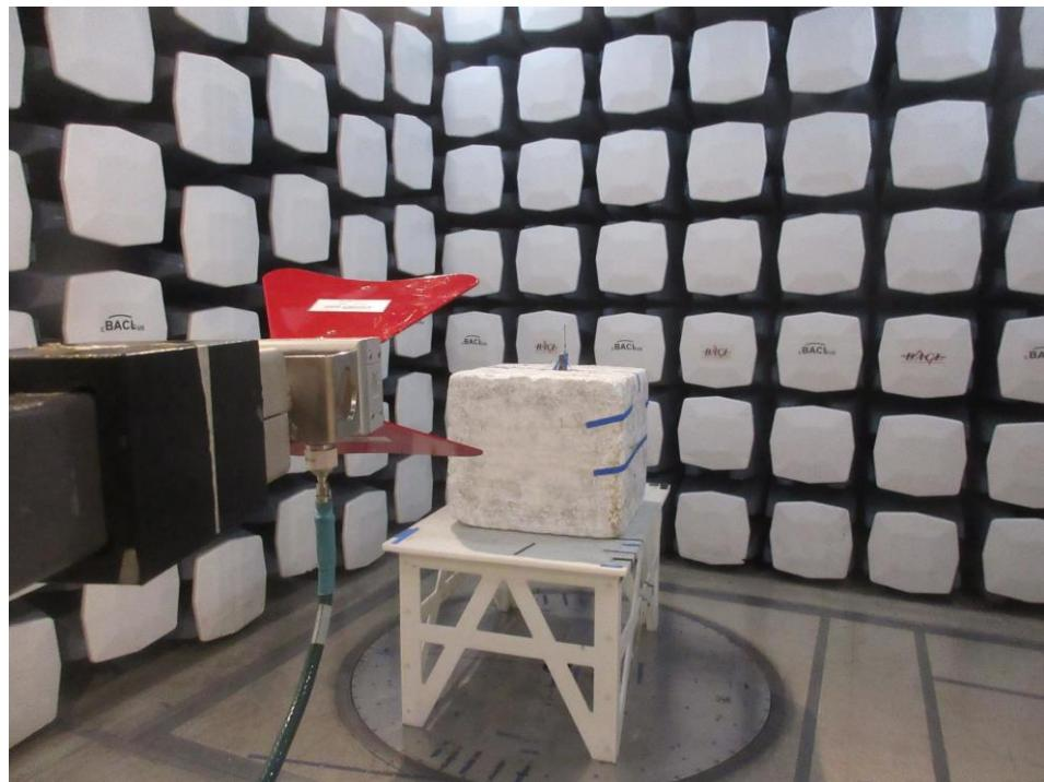
**1.8 Radiated Spurious Emissions: 1-18 GHz Rear View at 3 meters (Substitution Method)**
