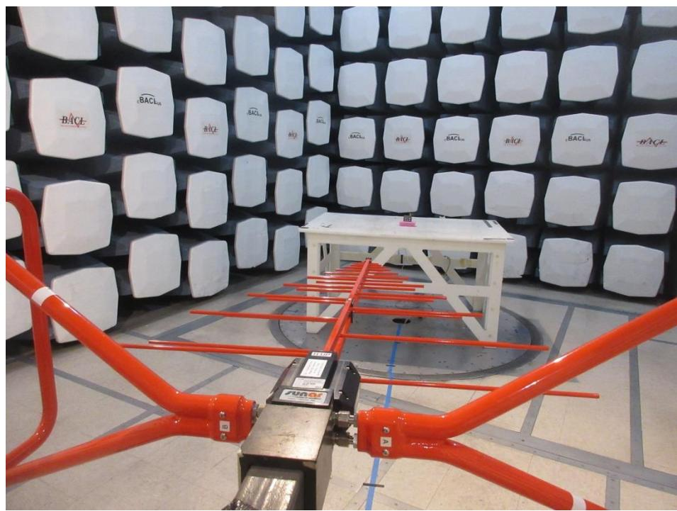
**1.6 Radiated Spurious Emissions: 30MHz - 1GHz Rear View at 3 meters (Vasona Scans)**
