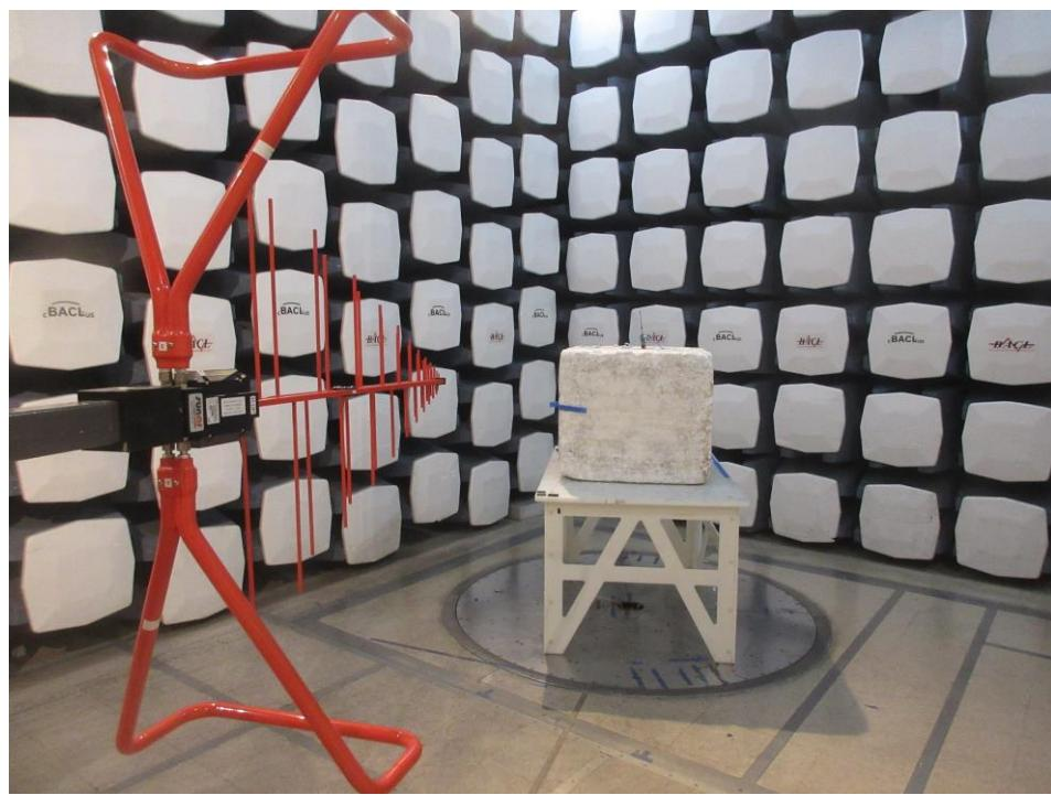
**1.4 Radiated Spurious Emissions: 30MHz - 1GHz Rear View at 3 meters (Substitution Method)**
