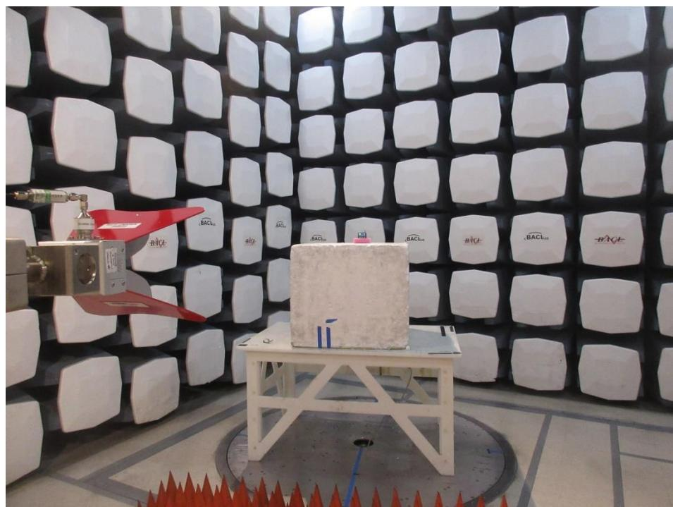
**1.10 Radiated Spurious Emissions: 1-7 GHz Rear View at 3 meters (Vasona Scans)**
