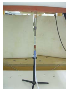
2450MHz System performance check setup
