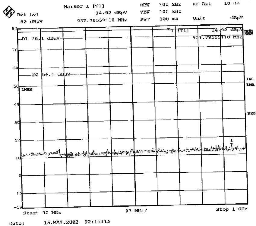
**Out of Band Emission(Conducted) :Tx(Ch11:2462MHz)1GHz-3GHz**
