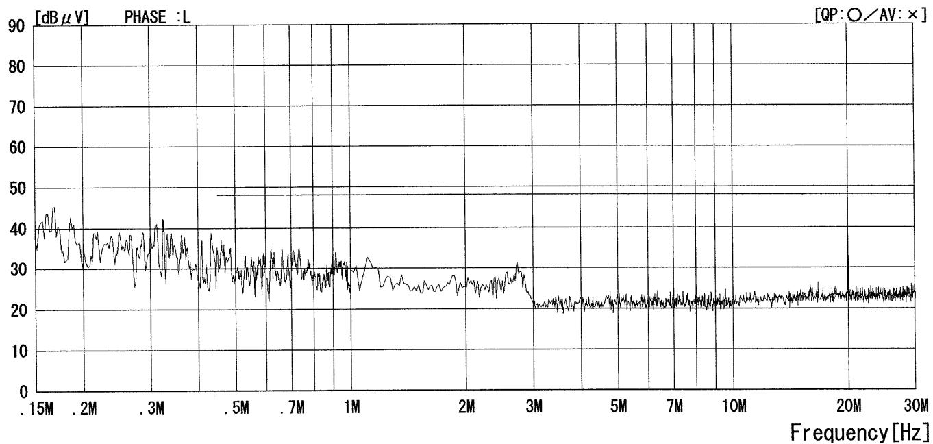
CHART : WITHOUT FACTOR , CALCULATION : RESULT=READING+C. F (LISN LOSS+CABLE LOSS)
