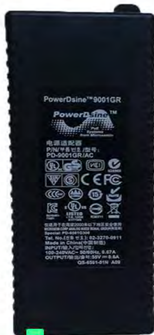
Figure 43: Microsemi® PD-9001GR/AT/AC PoE Front Panel
