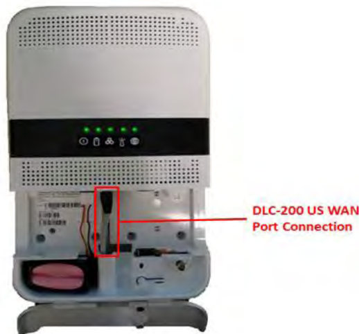
Figure 39: DLC-200C WAN Port Connection
