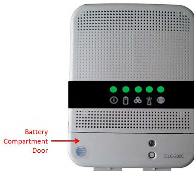
Figure 41: Battery Compartment—Front Panel
