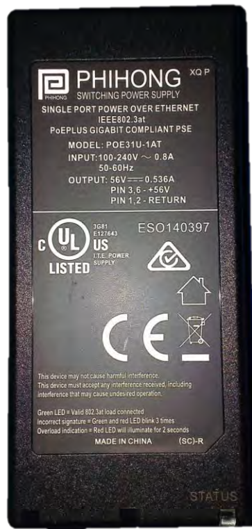
Figure 45: PHIHONG XQP POE31U-1AT PoE Front Panel
