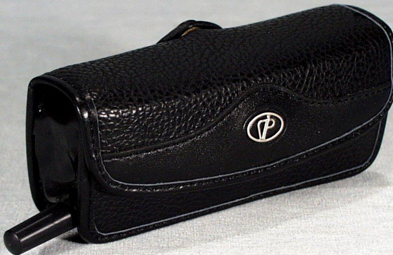
Fig.C-1 Photograph of the TECOM Model T-2000A placed in the holster. The metallic clip is on the opposite side which ensures that the antenna is angled away from the body in the body-worn configuration.
