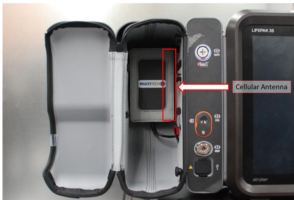
Photo 1-2 View of Cell Modem Inside Left Bag
