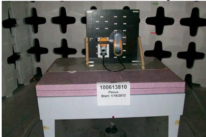
Axis 3 – Product Vertical & Rotated 90 Degrees
