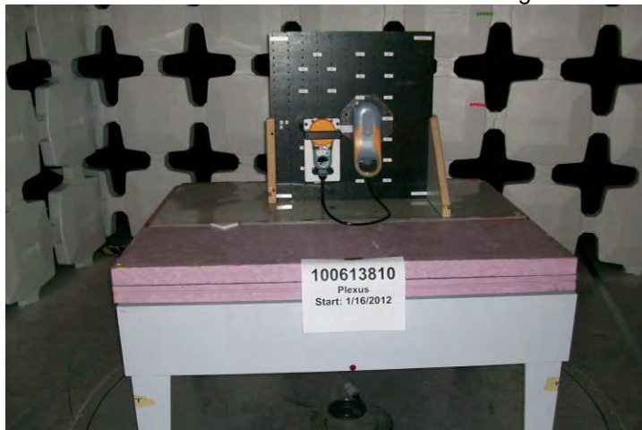
Axis 3 – Product Vertical & Rotated 90 Degrees
