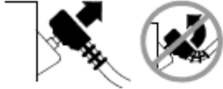
Figure 5-7 Disconnecting Defibrillation Cable from Test Post
