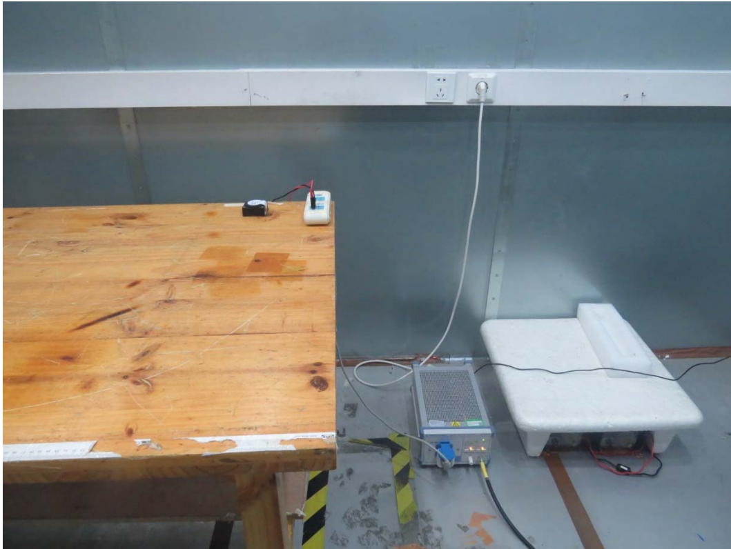
Picture 2 Conducted Emission Test Setup
