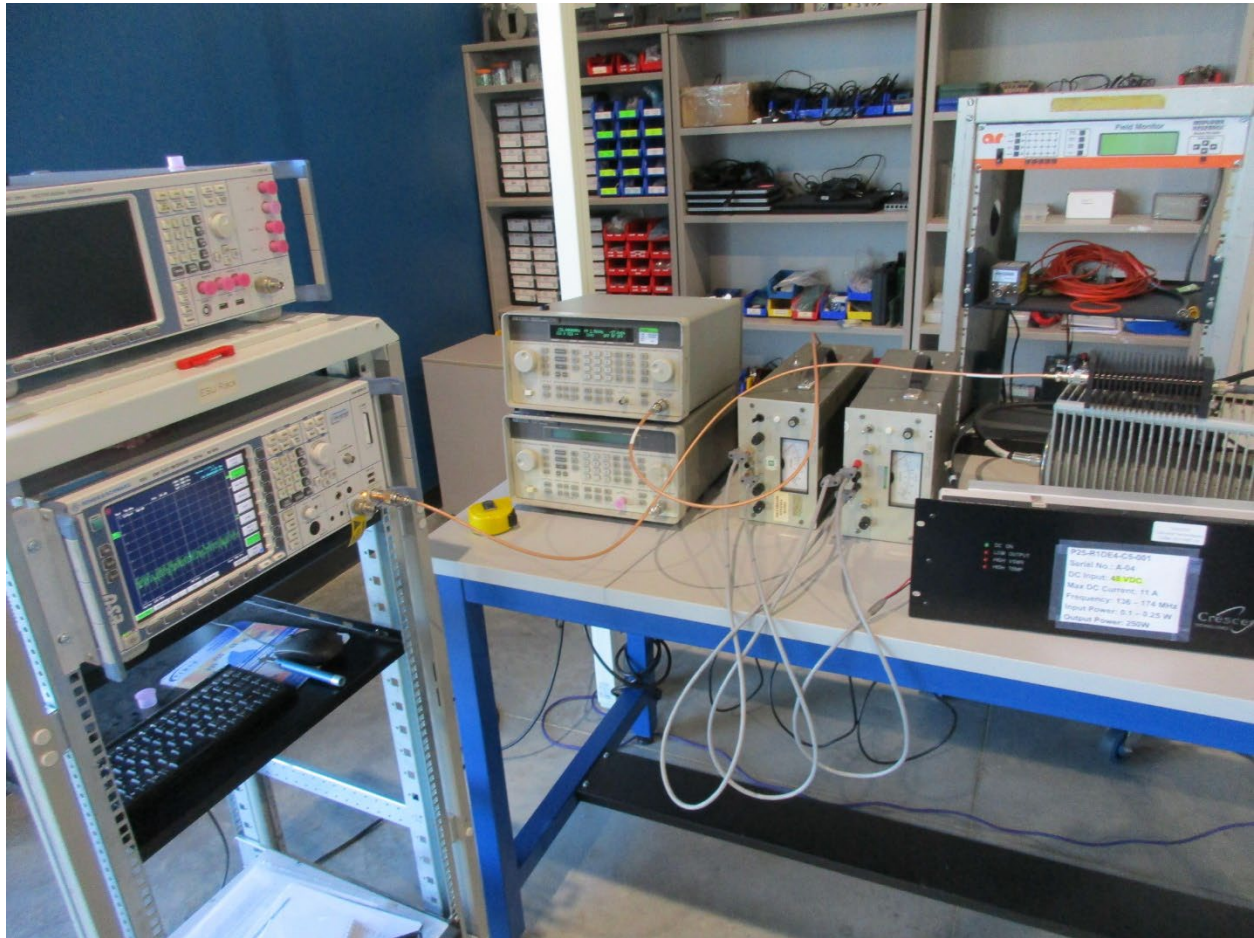
Conducted Test Setup
