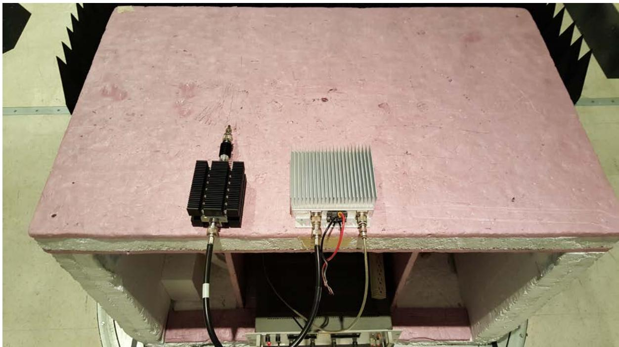
**FIELD STRENGTH SPURIOUS EMISSIONS – 9 kHz – 30 MHz**
