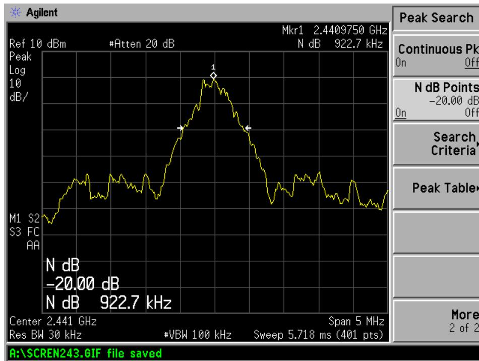
Result data graph shows 20 dB bandwidth, CF = 2.480GHz, BW = 0.898MHz
