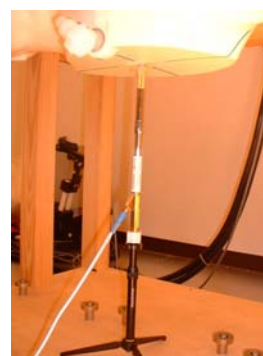
2450MHz System performance check setup
