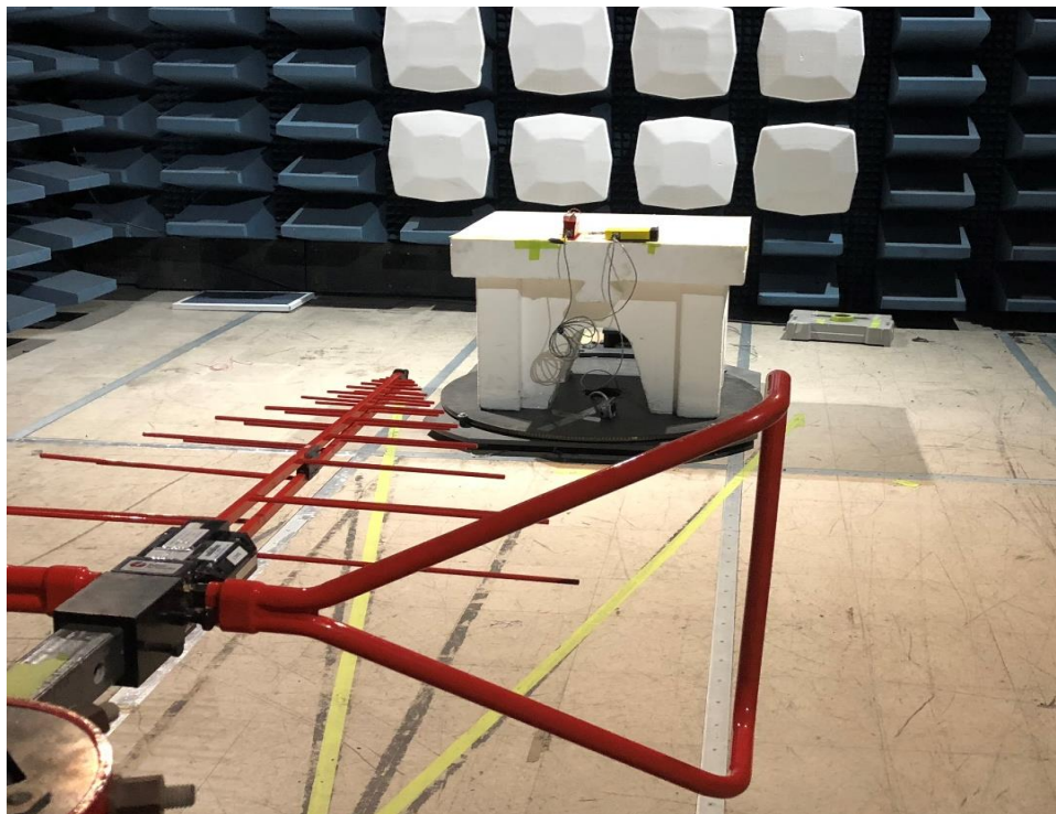
Radiated Emissions performed at the 3m SAC, 30MHz – 1GHz
