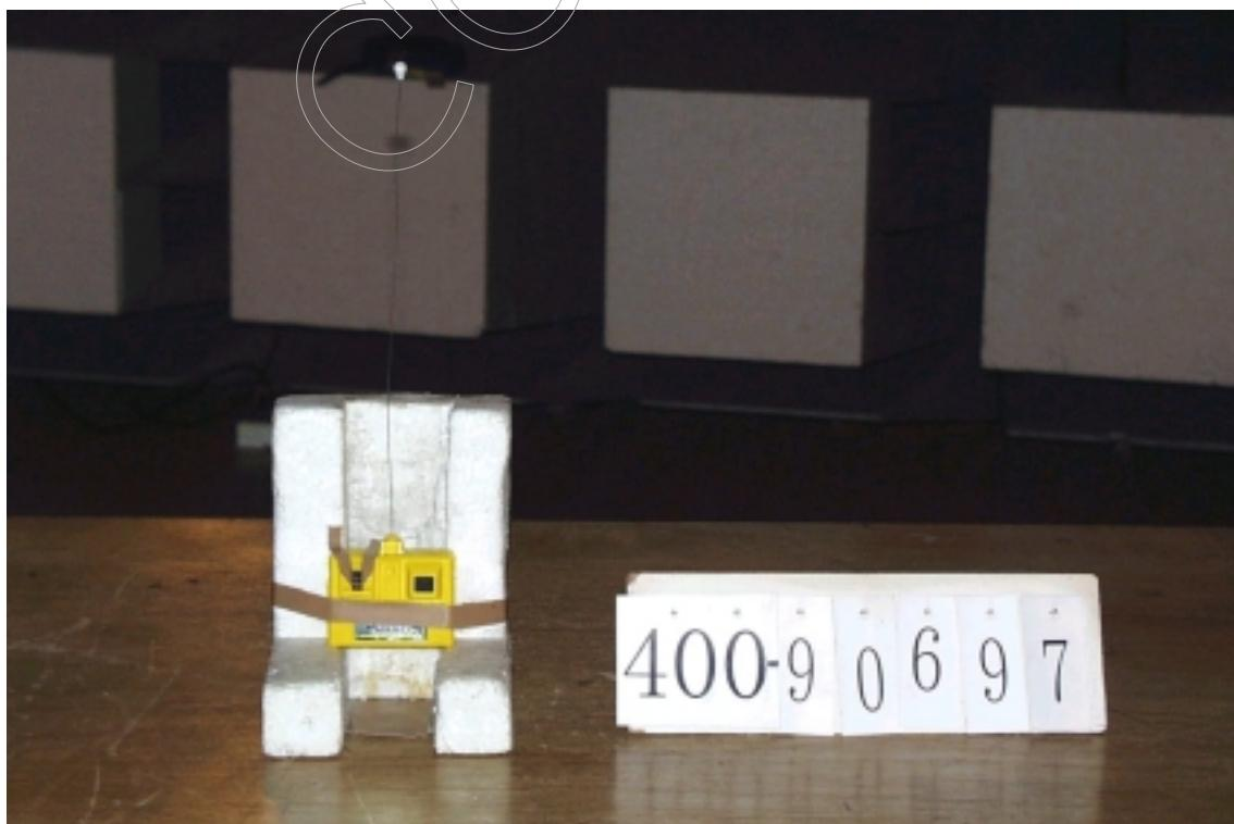
**TEST DATA****2.2 Radiated Emissions Measurement**Date : February 2, 2000Temp.: 20 °C Humi.: 40 %
