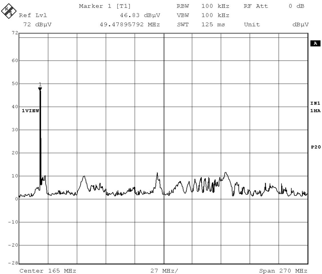
**2.3 Antenna Conducted Power Measurement**
