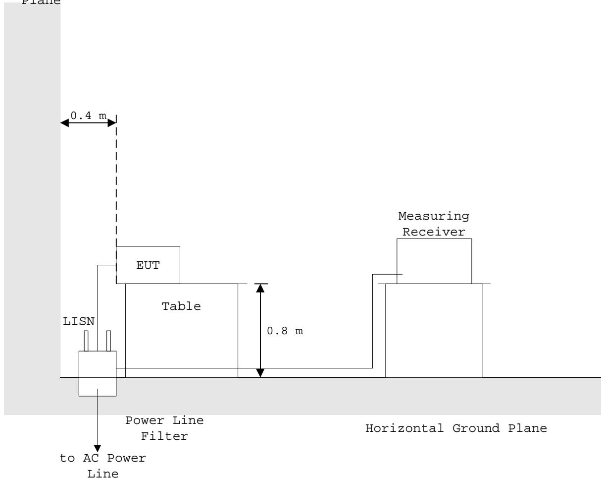
**1.8.2 Radiated Emission ( 30 MHz - 1000 MHz) :**
