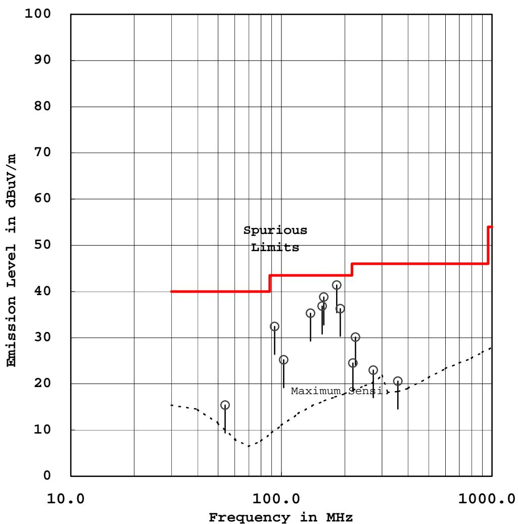
**Coherent Emission Plot**
