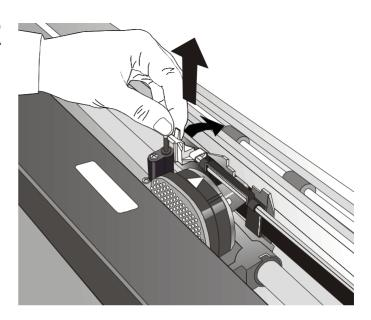
5. Remove the used ribbon cartridge by lifting it up.
