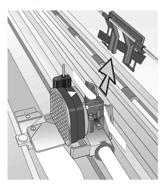
4. Free the shifter holder pushing the tab towards the rear and pulling the shifter holder up.
