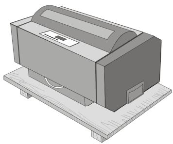
3. Insert the plastic bag over the printer and slide the packing box over the printer.
