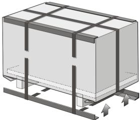
7. Fix the packing ribbon with the corresponding clips.
