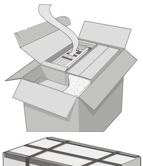
6. Close the packing box and fix it to the transport panel by means of the packing strip, inserting the plastic angles between the packing strip and the carton.
