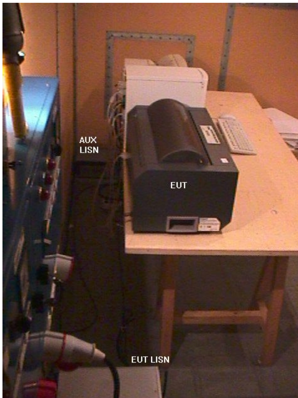
picture 6: conducted measurement rear view parallel transmission
