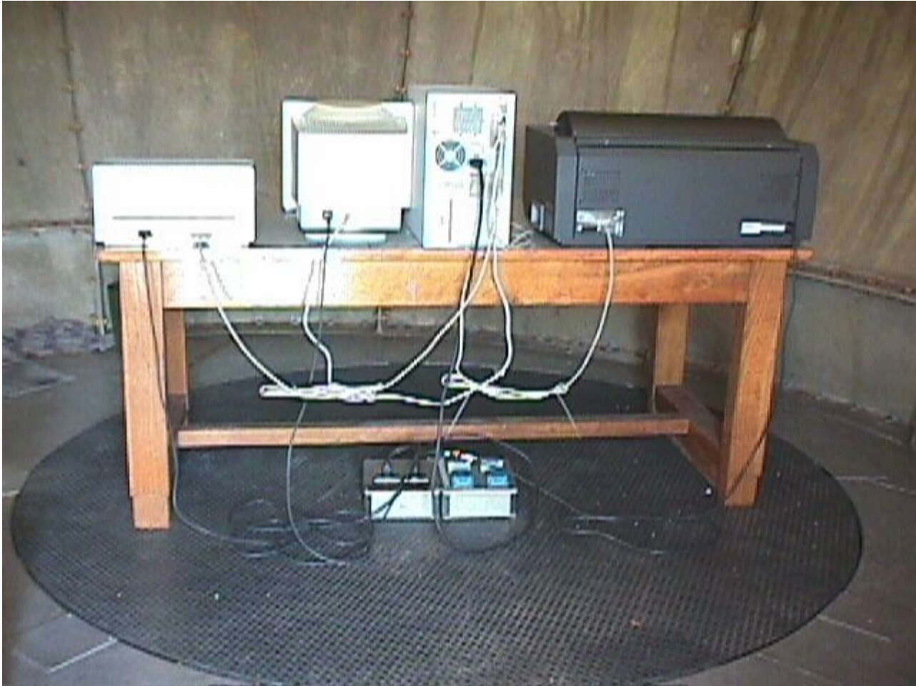
picture 2: radiated measurement rear view serial transmission
