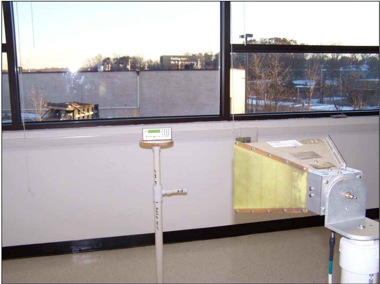
Photograph 2. Radiated Spurious Emission Test Setup
