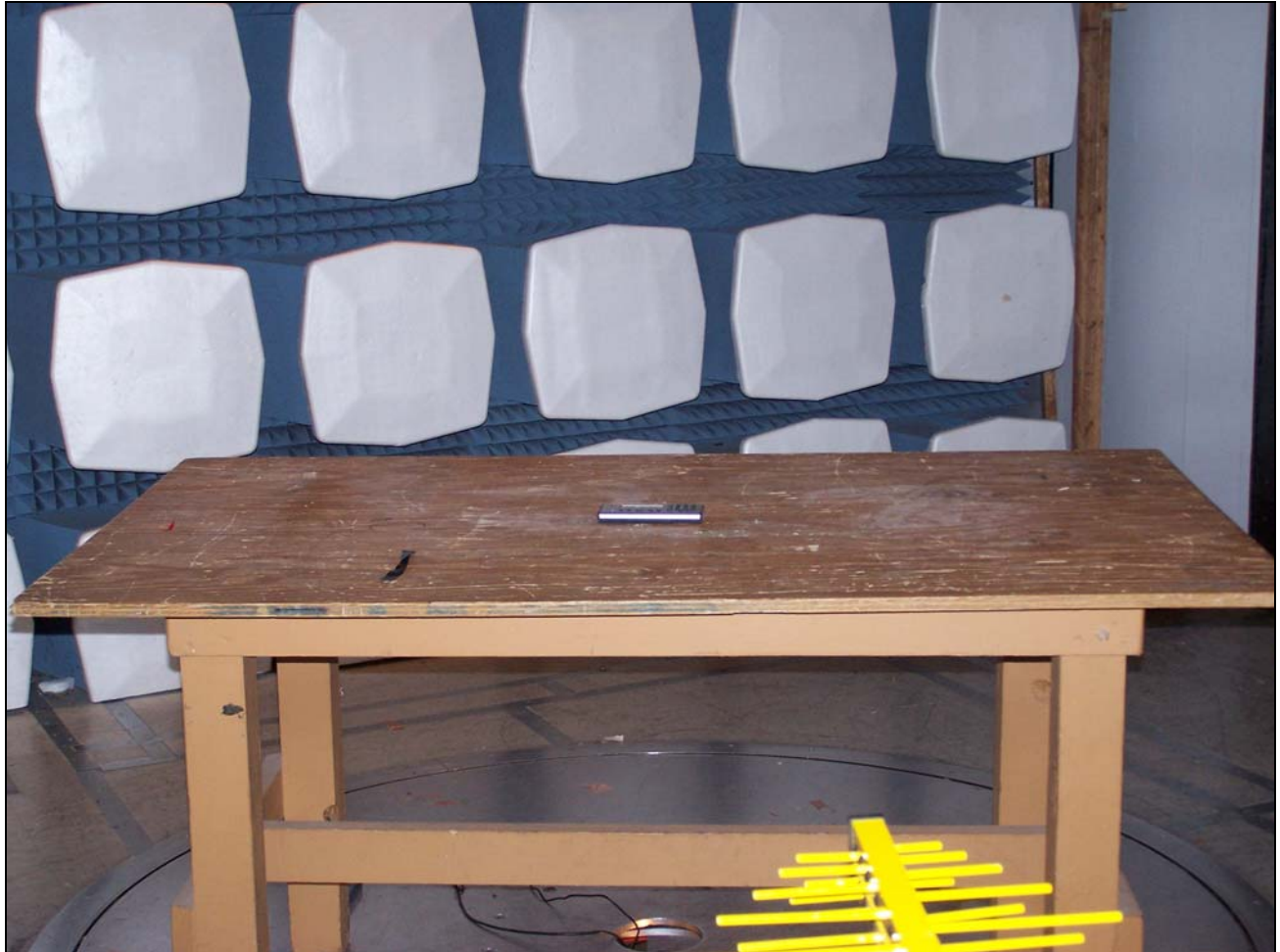
Photograph 3. Unintentional Radiators Test Setup
