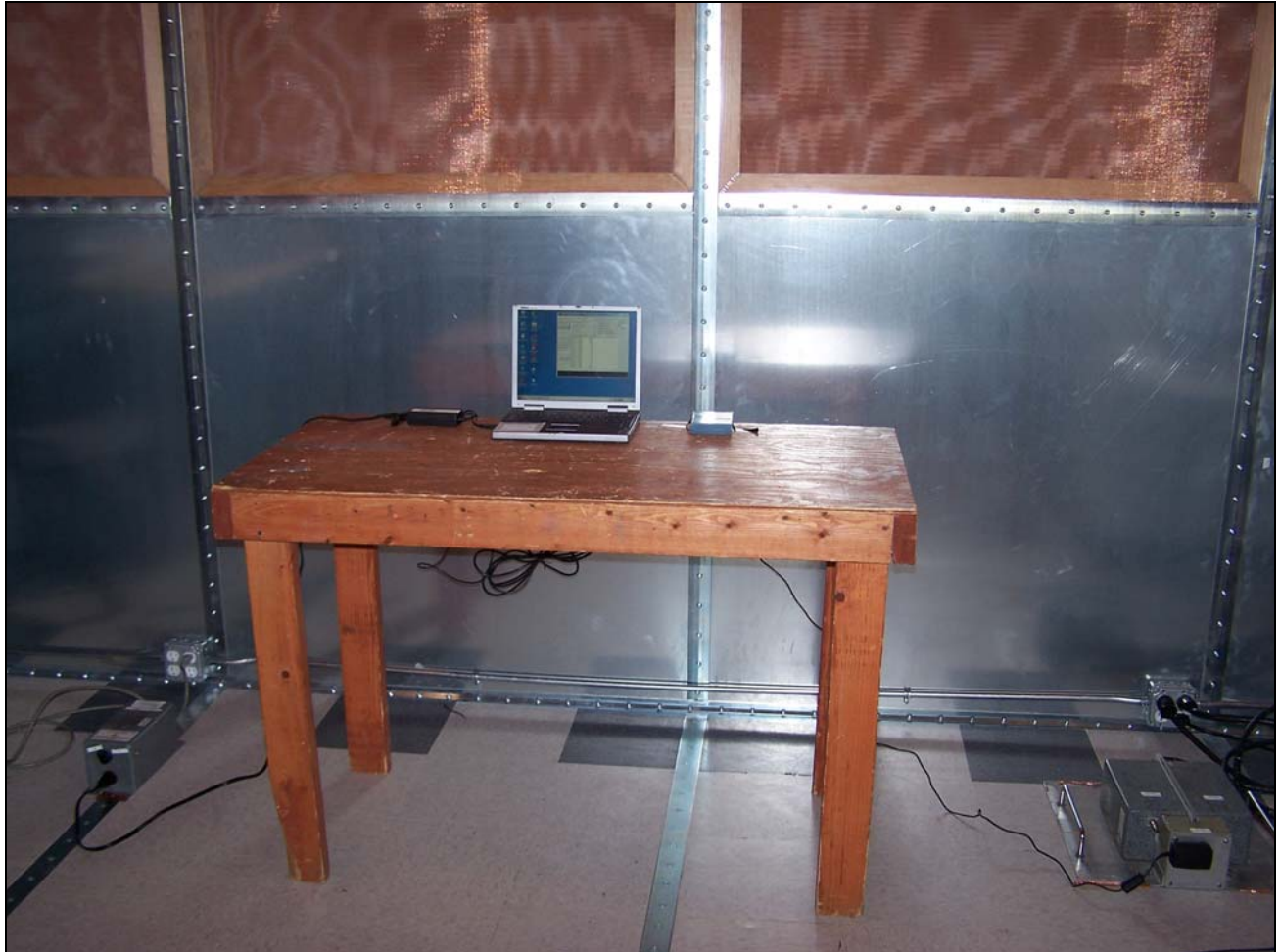
Photograph 2. Conducted Limits, Test Setup
