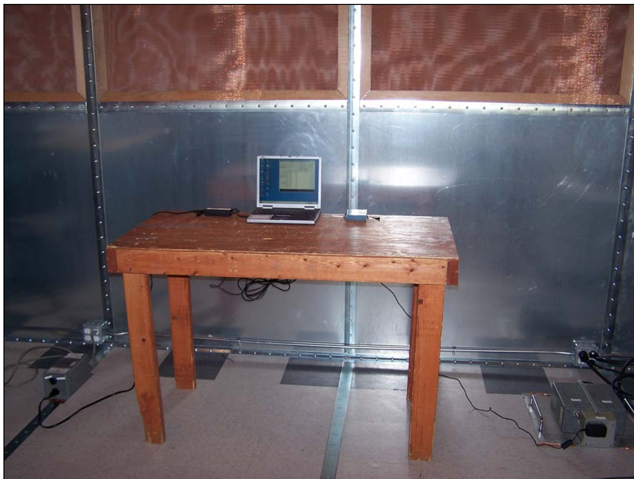
Photograph 1. Conducted Emissions Test Setup
