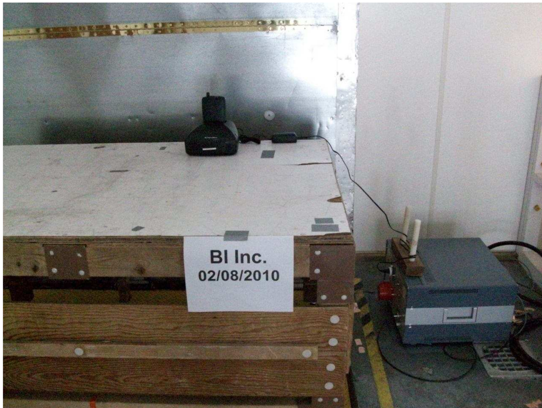
Conducted Emissions Test setup – Front View
