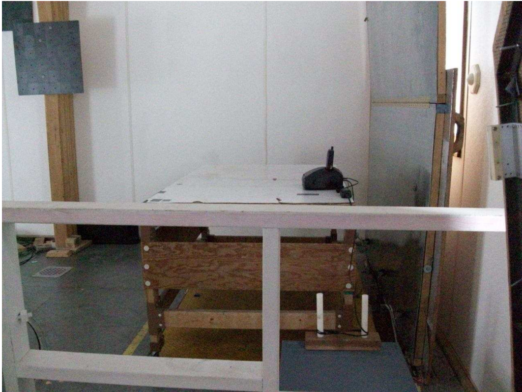
Conducted Emissions Test setup – Side View
