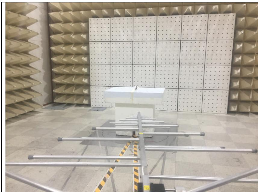
**3. Photo of Radiated Spurious Emission Test (Above 1 GHz)**
