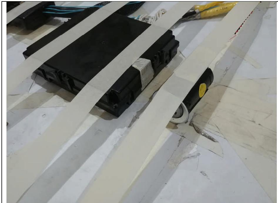
**2. Photo of Radiated Spurious Emission Test (Below 30 MHz)**
