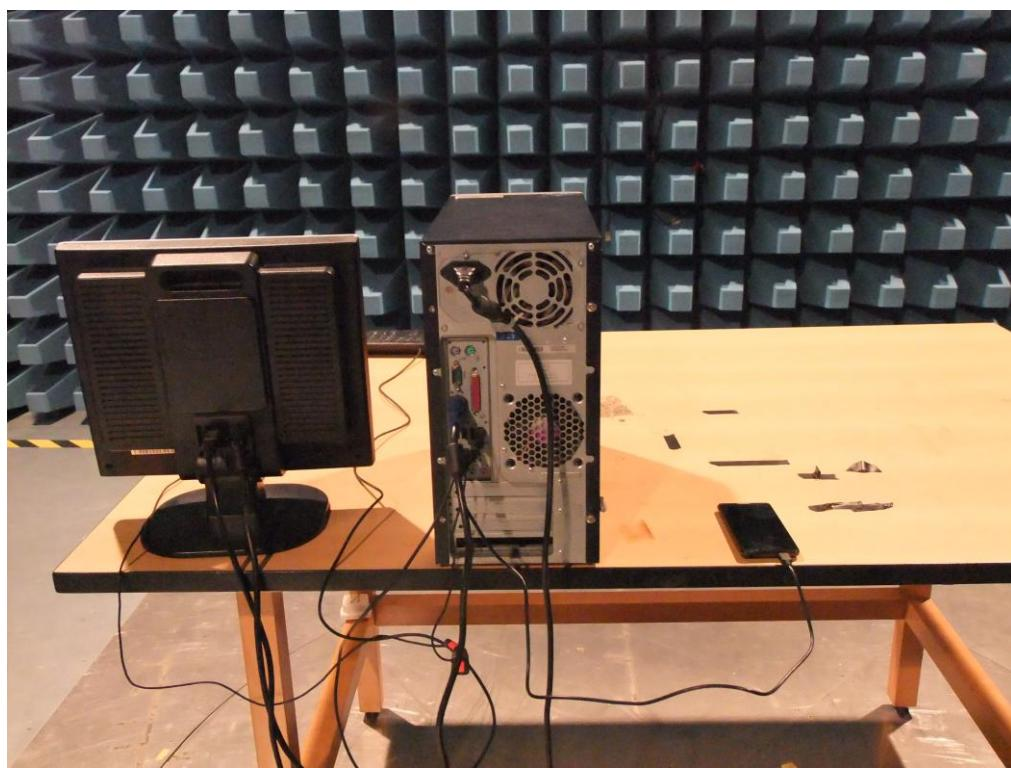
FCC Part15B Radiated Emission above 1GHz
