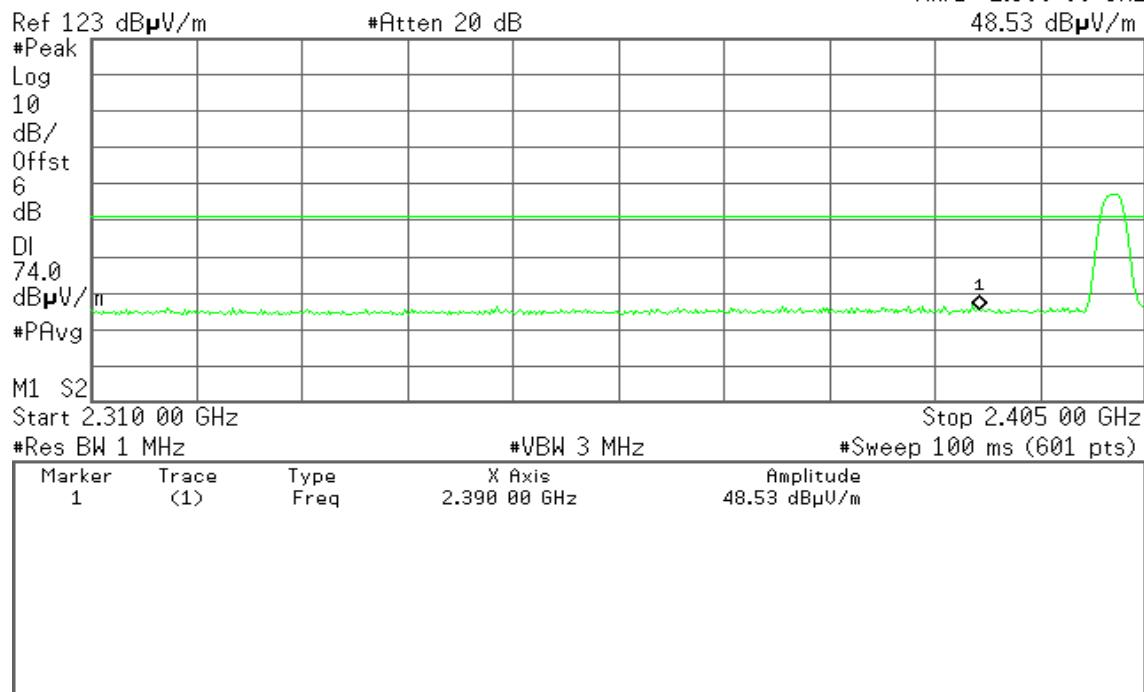
**Detector mode: Average****Polarity: Horizontal****Agilent**
