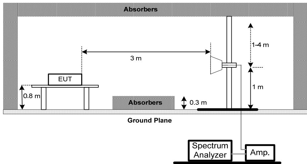
(C) For radiated emissions below 30MHz
