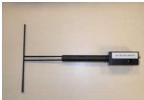
Figure 1 – Satimo COMOSAR Validation Dipole
