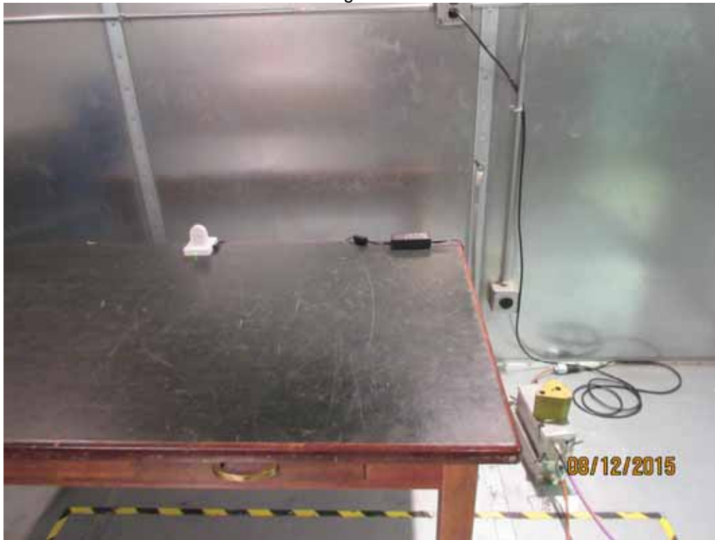
Test Setup for Conducted Emissions
