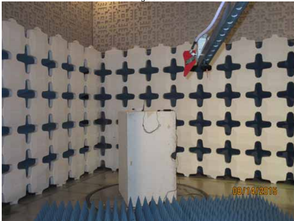
Test Setup for Transmitter Radiated Emissions – 1GHz to 10GHz, Horizontal Polarization
