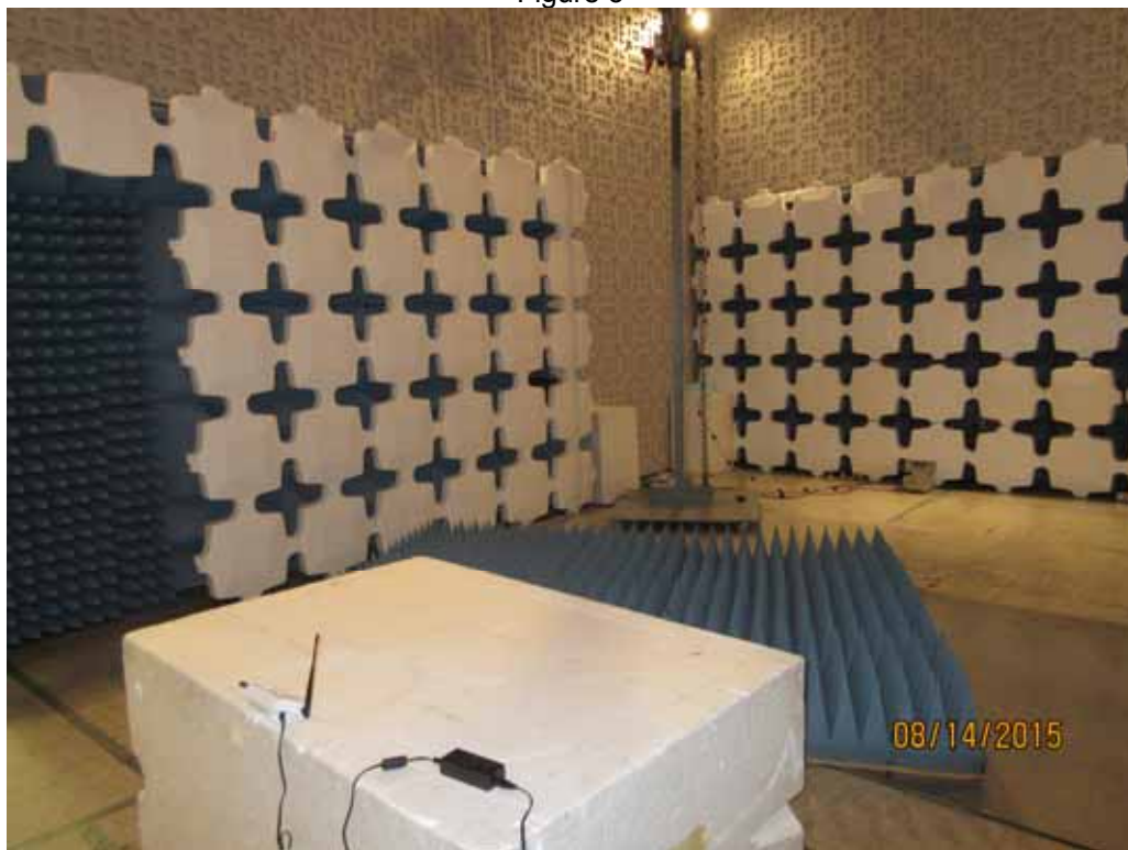
Test Setup for Receiver Radiated Emissions – 1GHz to 2GHz, Horizontal Polarization
