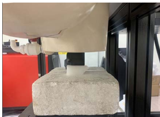
Fig.4 EUT Front tilt side to flat phantom
