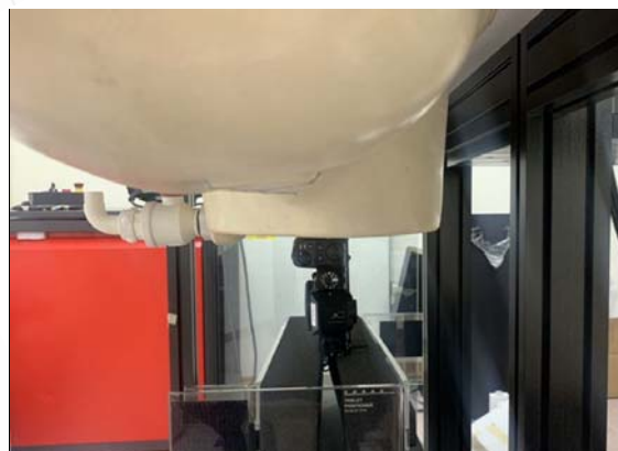
Fig.5 EUT Left side to flat phantom
