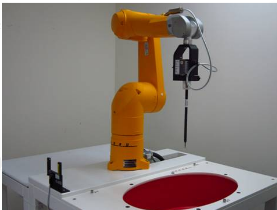
Fig.1 Photograph of the SAR measurement system
