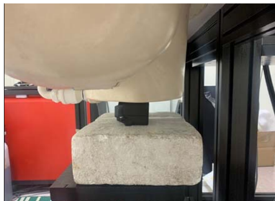
Fig.3 EUT Front side to flat phantom
