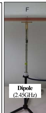
Test setup for the system performance check
