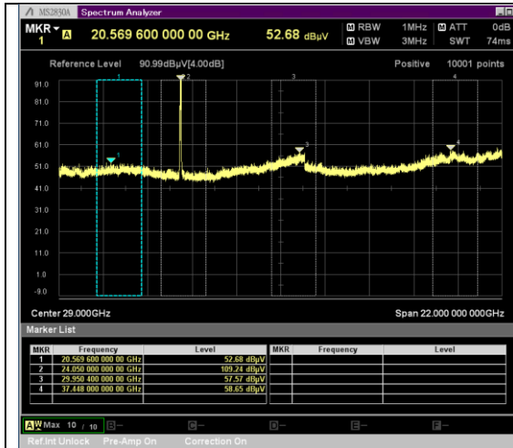
Radiated Emission 18-40GHz -Low (Peak)
