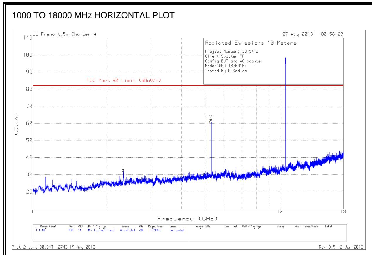
Note that the signal over the limit line is the fundamental frequency of the EUT
