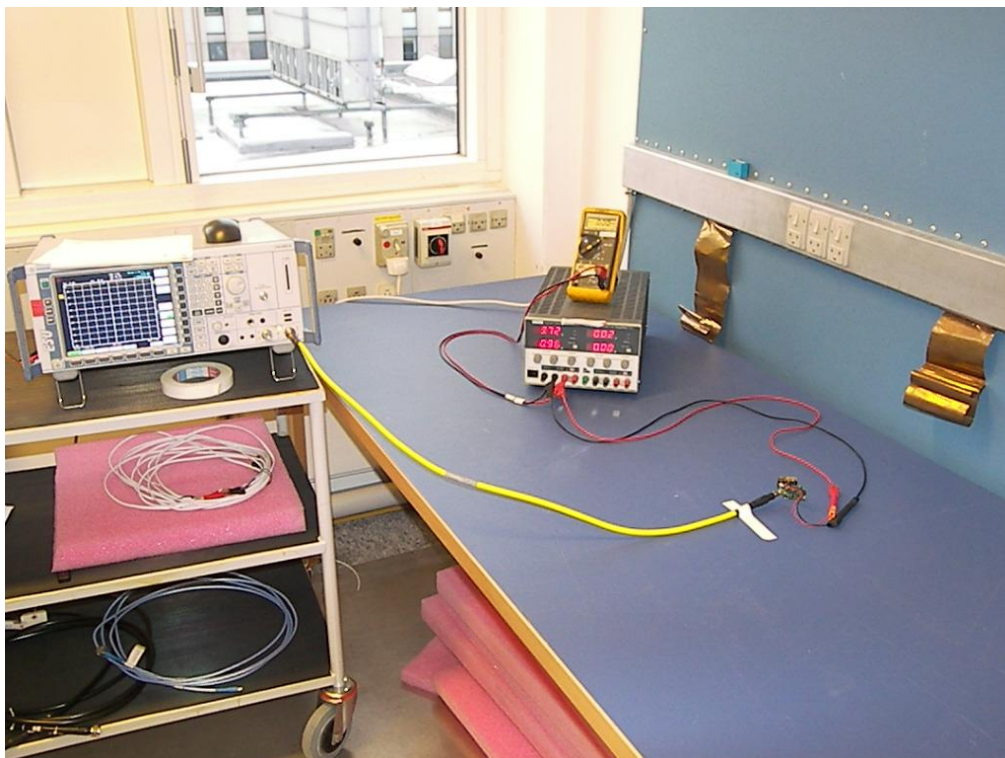
Photo Error! No text of specified style in document..13 Test setup regarding measurement of occupied bandwidth.
