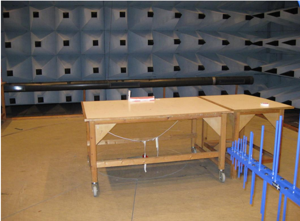
Photo Error! No text of specified style in document..2 Test setup regarding radiated emission, spurious, 30-1000 MHz.
