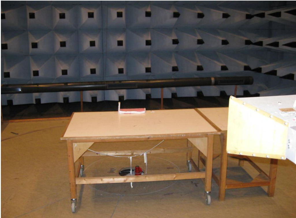
Photo 4.3.3 Test setup regarding radiated emission, spurious, 1-2.75 GHz.
