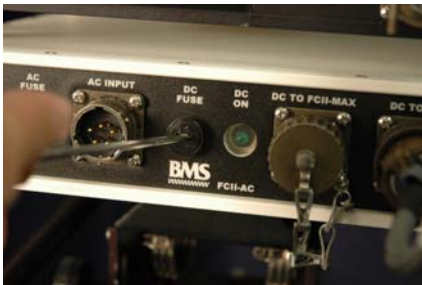
Unscrewing the DC Fuse Cap
