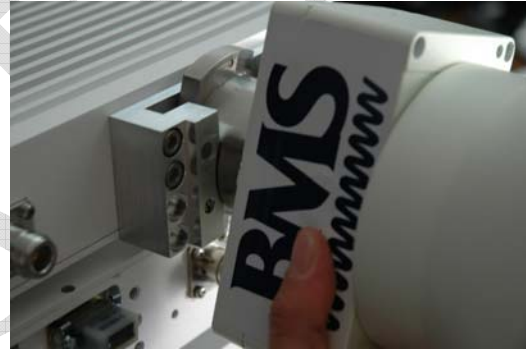
Figure 13 Insert Antenna Mount into Bracket
