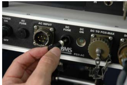
Removing the DC Fuse Holder
