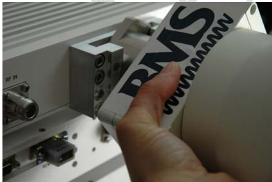
Figure 14 Rotate Antenna to Lock
