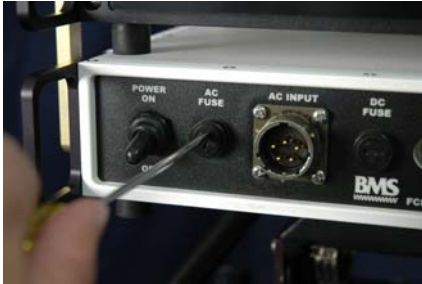
Unscrewing the AC Fuse Cap
