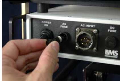
Removing the AC Fuse Holder
