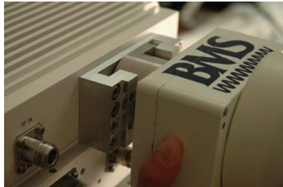
Figure 15 Antenna Locked to Mount
