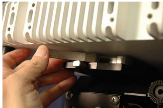
Figure 9 Fold the lever flush
