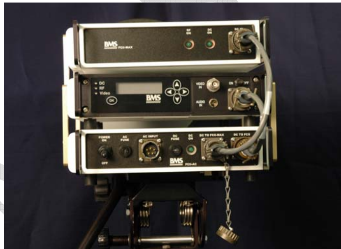
Figure 3 FCII-AC, FCII and FCII-MAX Attached Cable Connections
