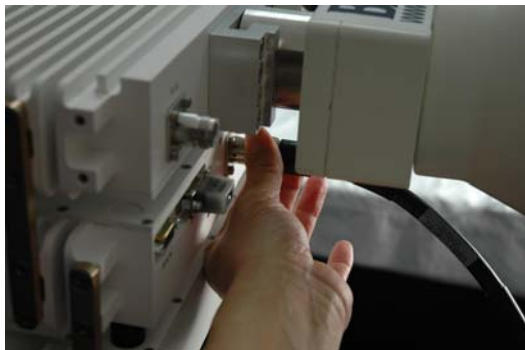
Figure 16 Connect the RF Cable to the FCII
