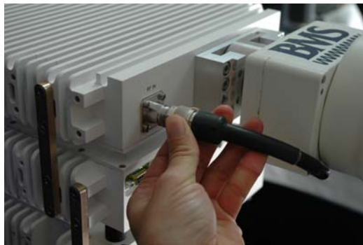
Figure 17 Connect the RF Cable to the RF In Connector on the FCII-MAX
