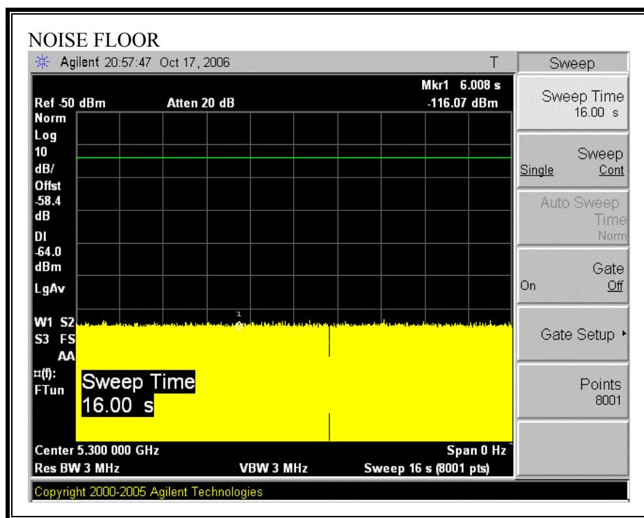
**PLOTS OF RADAR WAVEFORM**
