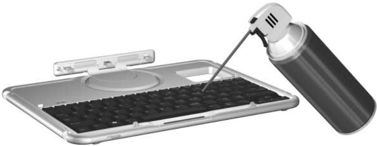
Cleaning a tablet PC keyboard with a can of compressed air
