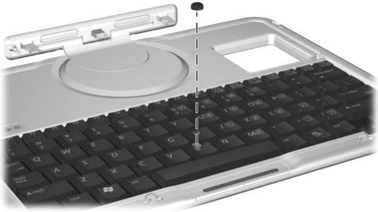
Replacing the pointing stick cap
