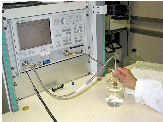
Tissue used during the SAR assessment is calibrated prior to use in the measurement process. APREL Laboratories use the co-axial probe method for all tissue calibration exercises. Tissue which is being used over a period of 24 hours is re-calibrated to ensure that no change to the dielectric properties will affect the SAR measurement process. The table below provides details of the results from the tissue equivalent dielectric calibration.
