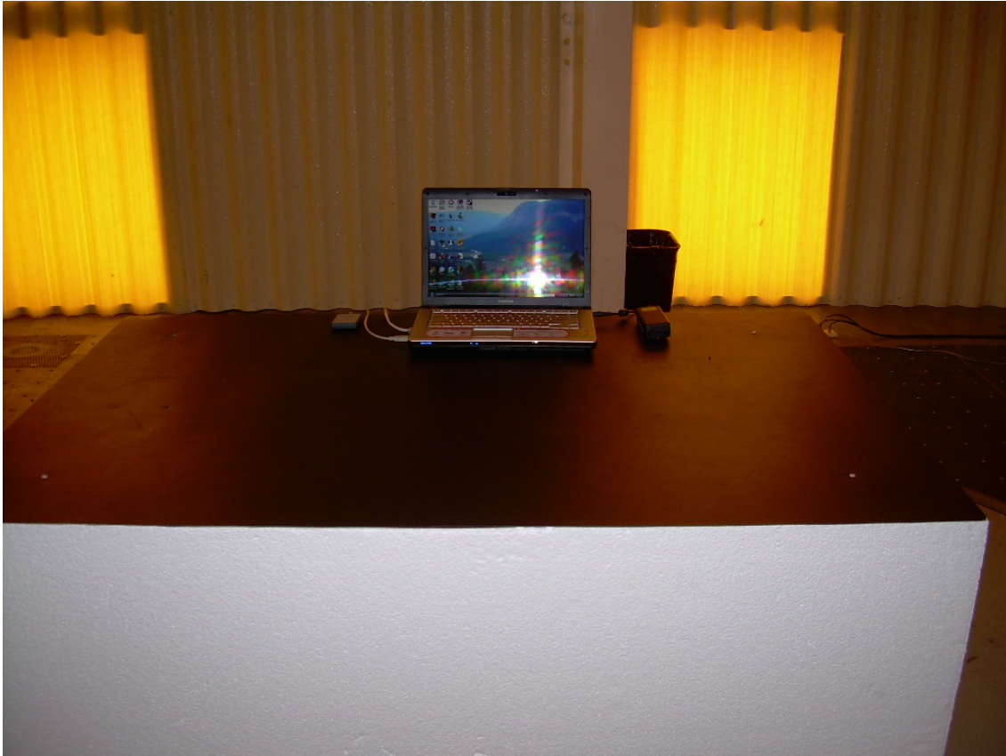
Photograph 1 - Front View Radiated Test Setup - Horizontal EUT Placement
